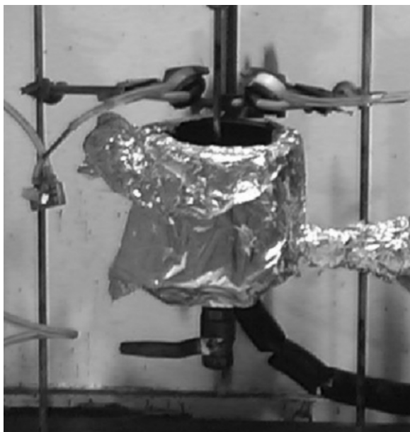
Fig. 2. Bitumen fume generation rig and sampling devices.
